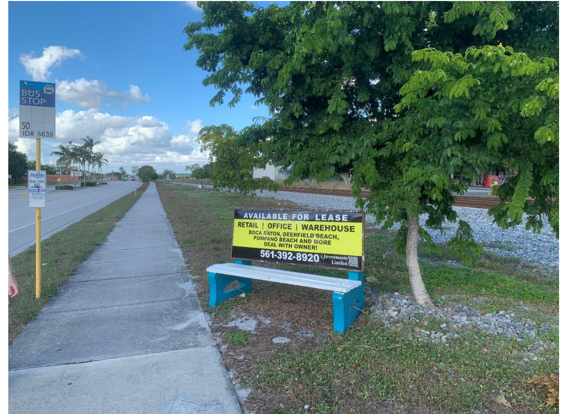
Missing boarding and alighting area
