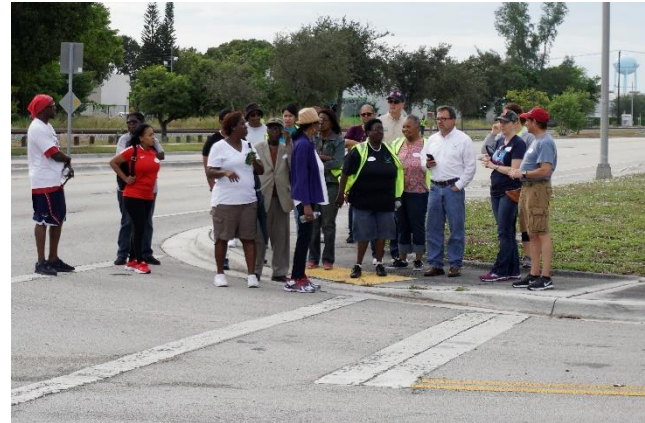
The width of the corner radii results in a longer crossing distance for pedestrians and allows for higher speed turns.
