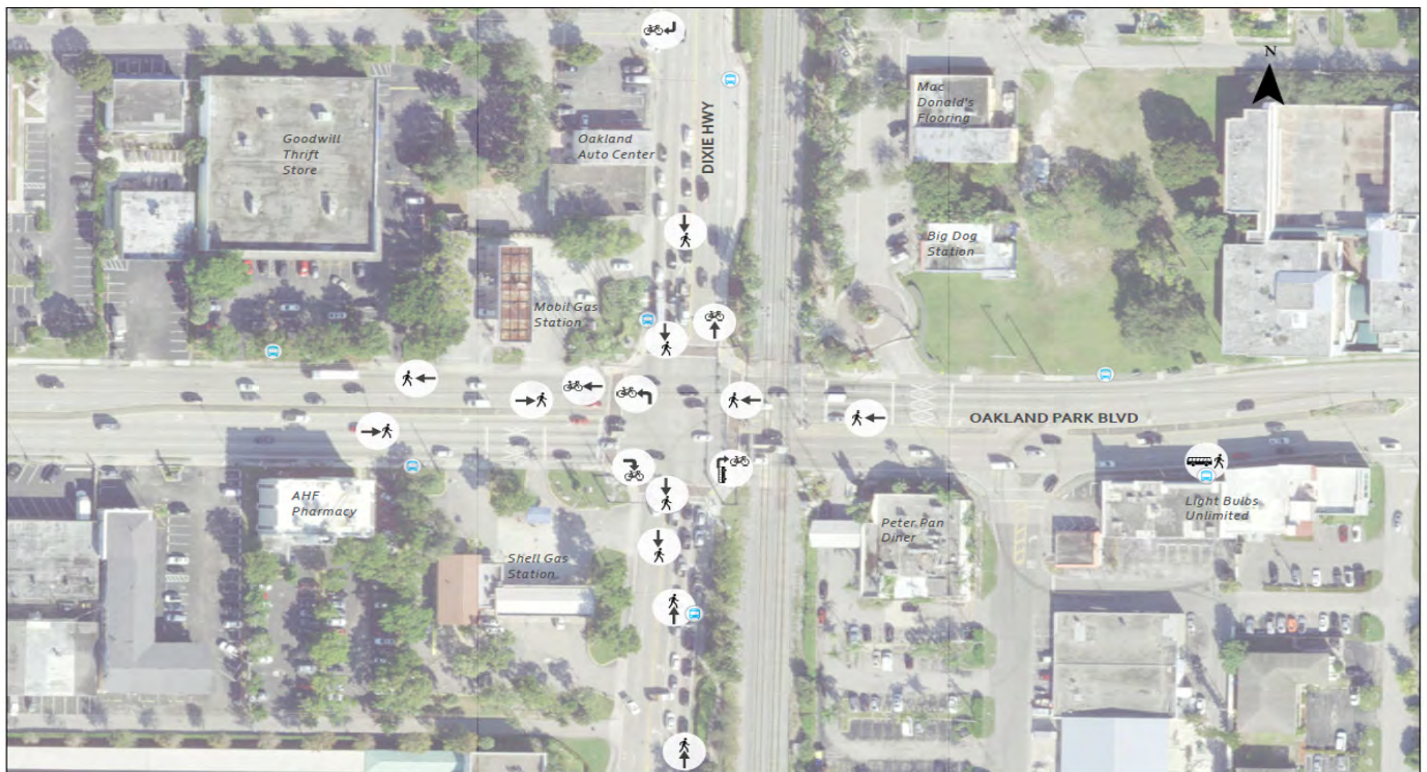
Figure 2: Bicycle and Pedestrian Crash Locations at Oakland Park Boulevard and Dixie Highway
