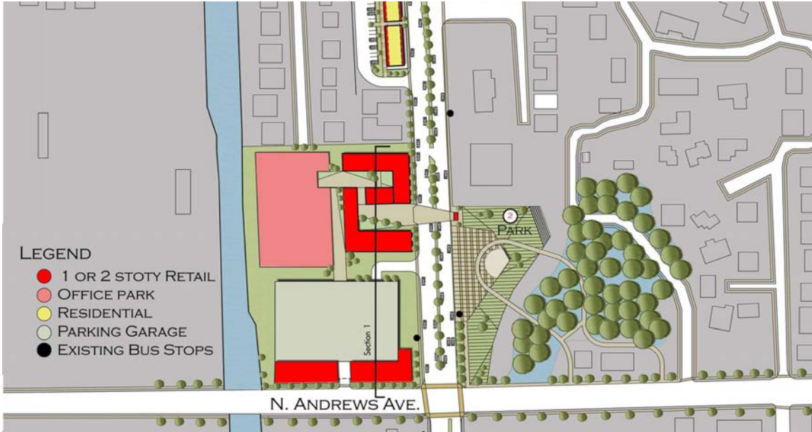
Fig 18a. Preferred area plans. Plan detail of 3 rd ranked scheme (Oakland Park Boulevard between Andrews Avenue and NW 9 th Avenue) from the first community scorecard event. The scheme features mixed uses on small parcels; predominant pedestrian circulation off of the main corridor; and enhancement of the access and use of existing waterways and landscapes. Source: FAU School of Architecture, Carlos Caceres and Jennifer Snyder. (Spring 2009)
