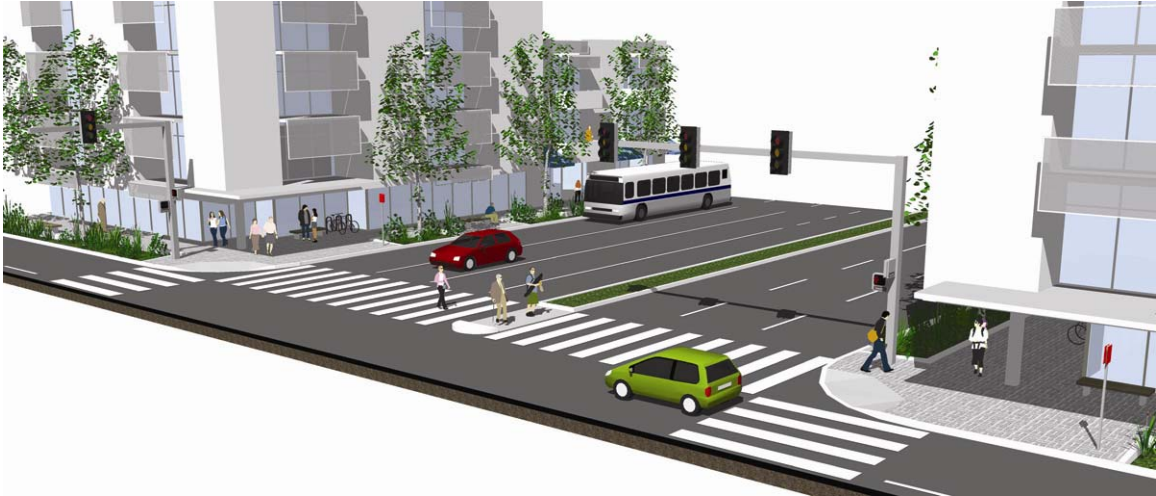
Fig 30. Accessible crosswalk typology with at grade surface treatment at the curbed median and pedestrian signalization integrated with street signage. Note placement of vertical poles within the landscape zone of the ROW so as not to interfere with the pedestrian route. Source: Broward County CDG, Pembroke Road (between SR-7 and the Florida Turnpike), Miramar Demonstration Area, Anthony Abbate and Alex McManus (2007).
