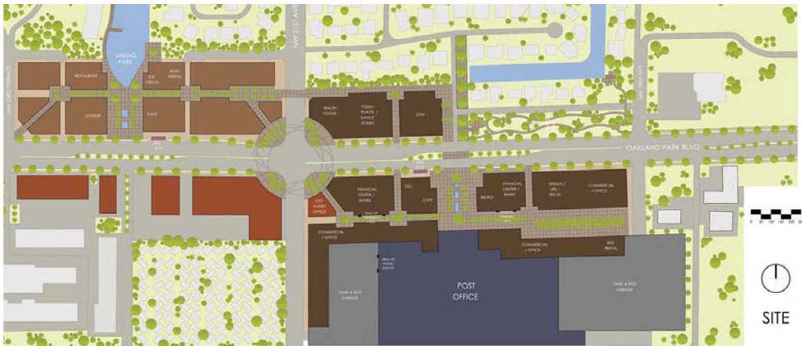
Fig 16. Preferred area plans. Plan detail of the highest rated scheme (Oakland Park Boulevard and NW 31 Avenue) from the first community scorecard event. Note the predominant pedestrian circulation (indicated in taupe) is off of the main corridor; pedestrian access to transit facilities is enhanced through the use of water features and shade trees; pedestrian and bicycle access is provided to nearby waterways. A circular form with corresponding crosswalk design creates a coherent urban space at the intersection with NW 21 Avenue.
