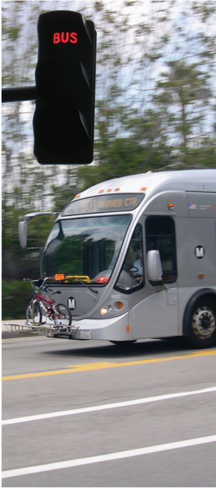
Rapid Bus features Traffic Signal Priority.
